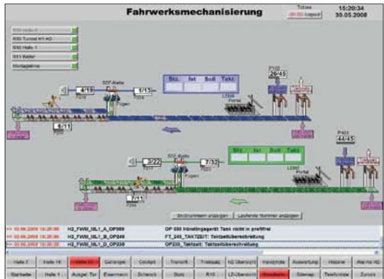
in Emden. The launch of a new model is usually also the event that triggers investment in new machines and software. Volkswagen in Emden took the production of the new series of Passat models as a trigger for modernising the assembly plant and standardising the base software as well as the overlaid visualisation software. Here, the zenon software from COPA-DATA, which is used for the central plant monitoring system, has been setting new standards in production.
