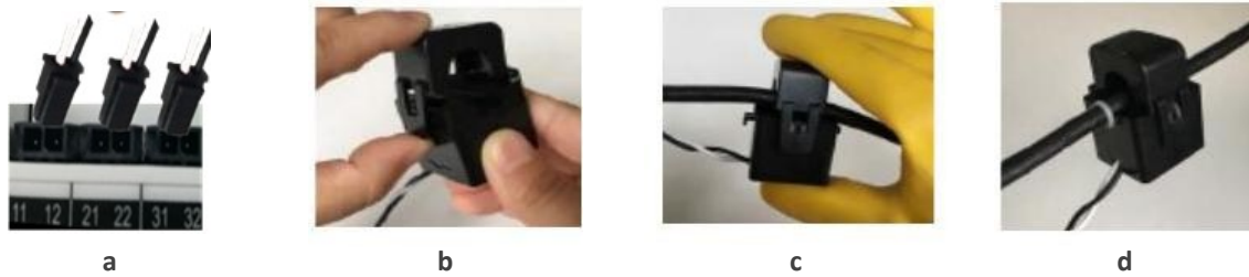
Figure 2-19 50A/40mA, 100A/40mA, 200A/40mA or 400A/40mA SCCT Installation
